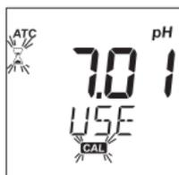
For better accuracy, frequent calibration of the pH sensor with the meter is recommended. In addition, the meter must be recalibrated whenever:
