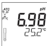
The LCD displays the pH value (automatically compensated for temperature) on the primary LCD, while the secondary LCD displays the sample temperature. If measurements are taken in different samples successively, rinse the probe tip thoroughly† to eliminate cross-contamination.
