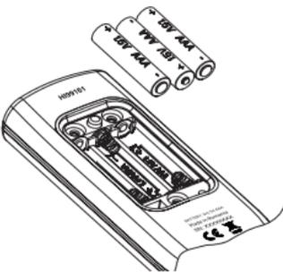
Replace the battery cover making sure that the gasket is in place.
