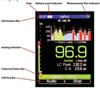
The Nova® uses a high resolution colour OLED screen to show a clear and easy to read display of all the information you need.
