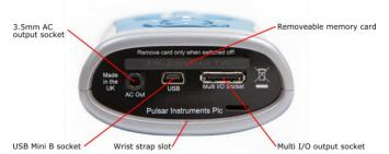
Install the AnalyzerPlus software on to a suitable PC and connect your Nova® to your PC using the supplied mini-B USB cable.
