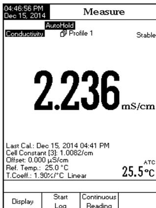
The United States Pharmacopoeia Regulations establishes limits and calibration requirements for WFI (Water For Injection). The HI5321 meter supports conductivity measurements that are needed for off line measurements in a Stage 2 of the regulation. Stage 1 verification may be carried out in a container but the regulation requires an in-line measurement. The meter provides prompts and instructions to make the measurements easily. Calibrate an EC probe prior to starting USP analysis.
