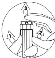
Figure 1: Removing Battery cover
