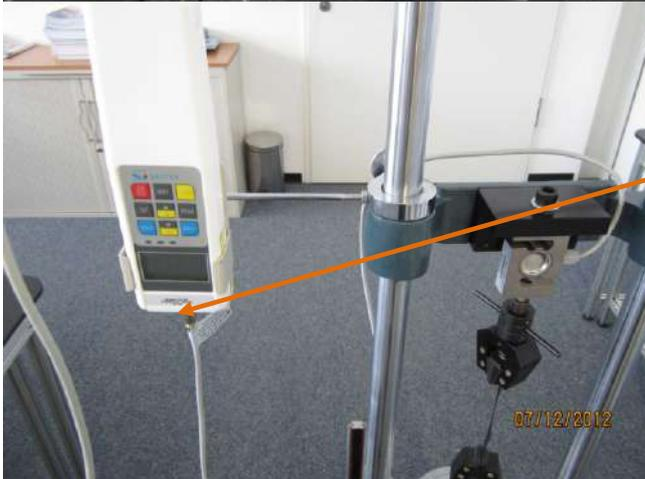
The plug of the external force gauge measuring cell has to be plugged into the socket of the FH force gauge.
