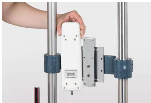
Tighten the force gauge with an Allen key M3 at all 4 screws M3x8 (screws are included in delivery of the force gauges)
