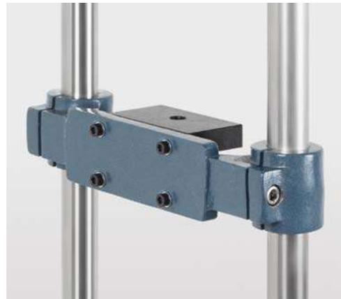
The external force measuring cell has to be mounted at the fitting bracket AFM 41 with a M12x40 screw (at TVS 5KN and 10KN) and with a M12x80 screw (at TVS 20KN, TVS 30KN and TVS 50KN), included in delivery.
