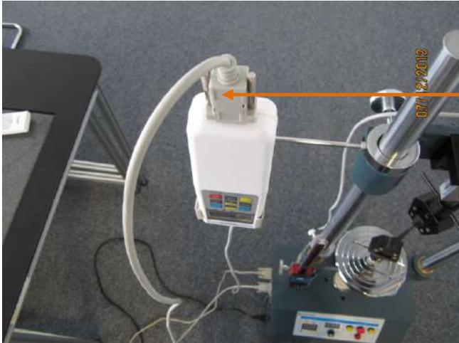
View from above FH with FH-A01 cable. A plug has to be inserted into the socket of the FH, the other one into the equipment port of TVS
