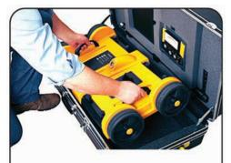
1. Remove the Base Unit from the carry case using the grab handles.
