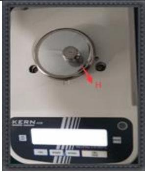
Move the weight to the lower-right corner (H) and record the displayed value of the balance. If it is a positive value, rotate the adjust screw at Position 2 with socket clockwise. If the value is negative, rotate the adjust screw at Position 2 counterclockwise.
