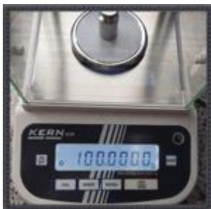
Put a 100 g weight (half the capacity of the balance) on the center of the weighing pan, read and record the displayed value.
