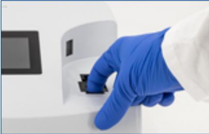
Fig. 5: Remove cuvette adapter
