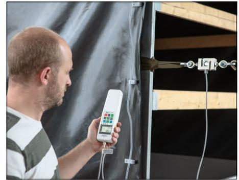
Universal digital force gauge for tensile and compressive force measurements with external measuring cell
