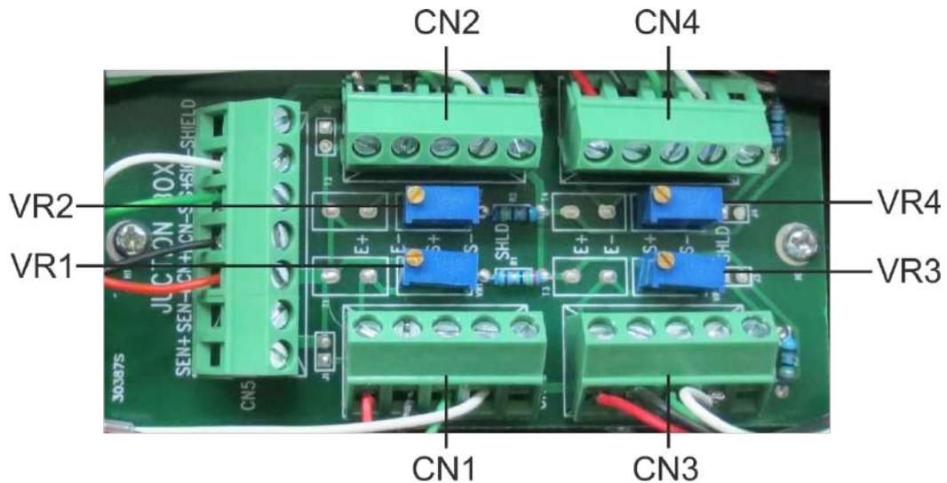
Adjustment of weighing cell CN1 takes place at the potentiometer VR1
