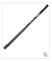
Introducing a frying oil monitor that can be used to periodically check and monitor the quality of oil. This instrument is capable of measuring both TPM (Total Polar Materials), a standard used in Europe as an indicator of the overall quality of frying oil, as well as AV (Acid Value), which indicates changes in cooking oil properties.
