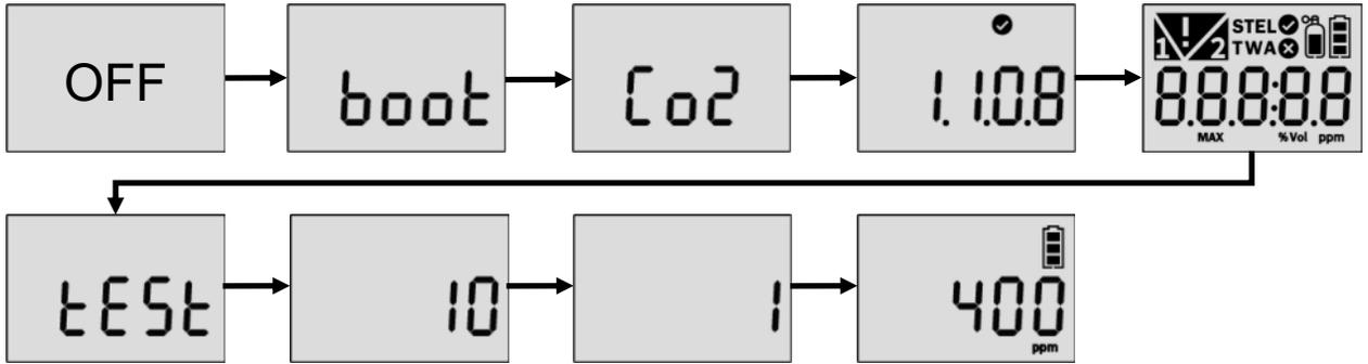
If the stabilization is failed, Error mark is displayed and measuring mode will not be entered. In this case, contact authorized resellers or SENKO service center at 82-31-492-0445 for repair or return.
