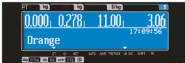
The LCD display is used for displaying 4 digits of tare value, 5 digits of weight value, 6 digits of unit price and 7 digits of total price. And the dot matrix LCD display is used for displaying commodity name up to 12 characters.
