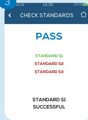
The check takes 10 seconds. If the instrument is functioning correctly, a PASS will display on screen and the corresponding line will turn green.
