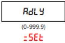
**Alarm Delay Time (Default: 0.5, Max: 16 min)**
