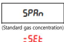
If you press the setting button once again while "SPAn" is displayed, the set calibration gas concentration is displayed as a number.
