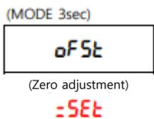
If the setting button is pressed for 3 seconds, "ofSt" is displayed, and if the setting button is pressed once more, the current concentration is displayed.
