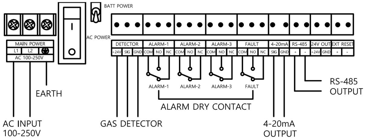
Connect AC power (100 - 250 V, 50/60 Hz) to the power as shown in the figure.
