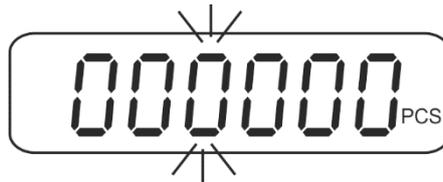
⇒ To enter the lower limit, e. g. 75 items, press the navigation buttons (see chap. 3.1); the currently enabled digit will be flashing.
