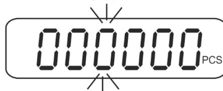
⇒ To enter the upper limit, e. g. 100 items, press the navigation buttons (see chap. 3.1); the currently enabled digit will be flashing.
