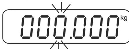
⇒ Press the navigation keys (See chap. 3.1) to enter the upper limit, e.g. 1100 kg; the currently enabled digit will be flashing.
