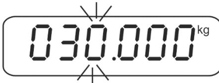
⇒ Either apply the displayed adjustment weight or make changes with the help of the navigation keys (See chap.3.1). Confirm by
